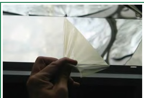
Step 7 - Remove all the yellow protective film from the inside of the Conversion Box.
